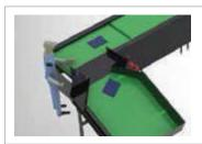
Take-off Conveyor - This is the single point entry of shipments in our DWS. It is meant to be used for bulk loading. This induction keeps in mind the principles of ergonomics and makes sure that minimum strain is caused to the operators.
