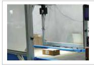
Weighing - Our special weighing conveyor is a rugged yet sensitive conveyor designed to handle items of different weights, but providing the same level of precision and accuracy while in motion!
