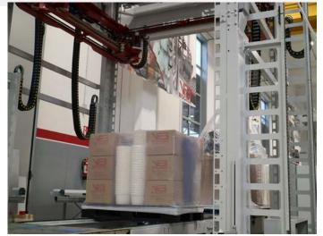
The FB3000 stretch hood machine is designed to offer flexible packaging standards.
