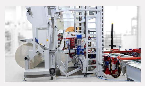
All machine maintenance is done at **operator level** to grant the **upmost safety**. A patented system allows to **lower the top frames** of the machine individually or separately.
