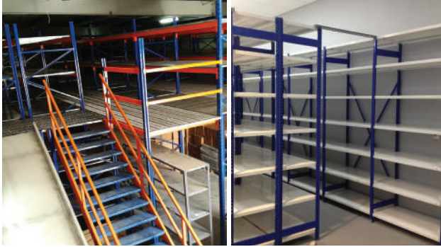
Mezzanine Racking / Shelving System
